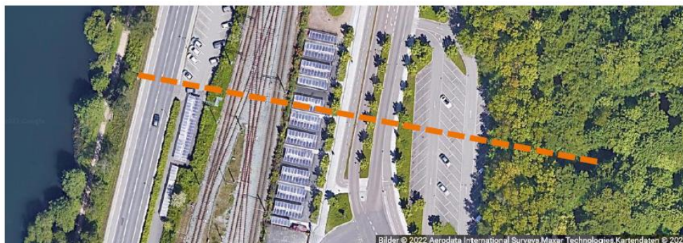
Figure 18. Run of the sewer pressure pipeline under Holte train station
